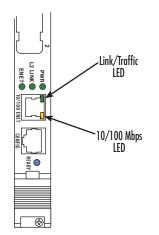
Figure 3. Model 6081RC Ethernet port LEDs
